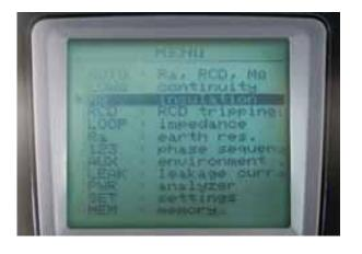
General menu to quickly selection of available test performed by meter (COMBI419 and COMBI420 models only)
