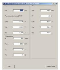
Final result of a PV test performed with SOLAR300N and downloaded by TopView software. Possible export in XLS and PDF format files
