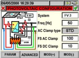
A synoptic connection scheme on the display helps the user while connecting the instrument to the installation (Single or Three phase) under test
