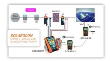
SOLAR300N performs all tests on PV plants by using of SOLAR-02 remote unit which, after a preliminary synchronisation, save in independent way the values of irradiance and temperature. Only at the end of test the remote unit should be connected again with the master unit to download the recorded data
