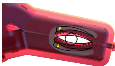
Megger clip being tested with IEC standard test finger for creepage and clearance.
