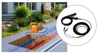
The Easyclamp transmitter clamp is used to send the 33 kHz signal onto and along live cables without shutting off their power. The Easyclamp is connected to the Easyloc TX transmitter and installed around the cable, providing effective route tracing.
