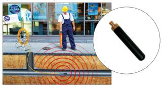
The MLS 55-3 pipeline transmitter probe is a slim, battery powered mini-transmitter and has a range of 5 m. When attached to a drain rod or fibreglass push rod cable by one of the 3 adapters provided, it is used to locate ductworks or blockages. A heavy duty protective cover is available.
