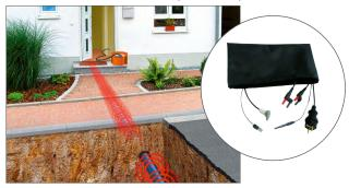
With the Easyloc house connection set, you can quickly and easily track the services leading from the house to the main line. The set consists of connecting cables for standard 13 A safety electricity sockets, cable TV and telephone sockets. To send a signal directly to the house connection the transmitter is connected to the relevant socket.
