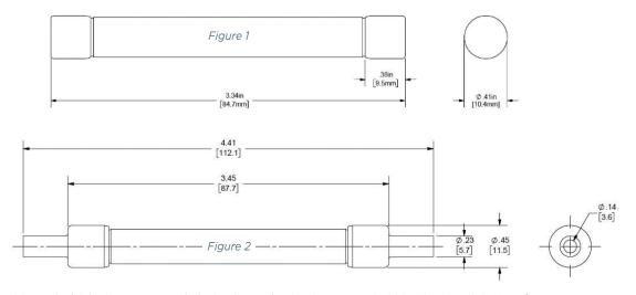
CC terminal (Fig. 2): Recommended crimping tool: T & B Sta-Kon ERG4002 #10 -12 AWG (6-4 mm²)
