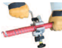
Cable sheath stripping
