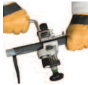
Scoring and removing Easy-Peel strippable semi-conductive layer
