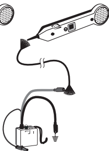
Figure 2b. Cable Tracing
