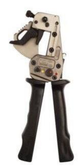
This copper flat band cutter enables mechanics to cut copper flat band up to ca. 0.24 x 1.57inches, (6x40 mm) at place. Through the low afford of force and its easy use, it is possible to use under narrow conditions. No more sawing! Quick blade release allows fast backout in any position. Can be used even in confined areas
