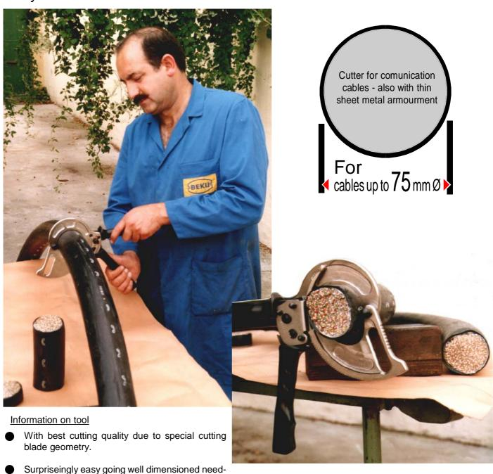
le beared movement mechanism (patented in germany and abroad)
