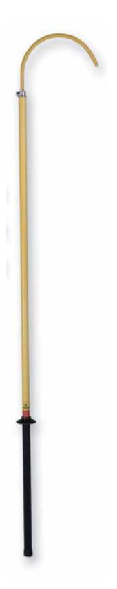
Poles with only one section, made of polyester and fibreglass tube  $\emptyset$  32 mm. With humidity-proof seals on each end, hand protector, grip, tip, M-10 metric head and rescue hook.
